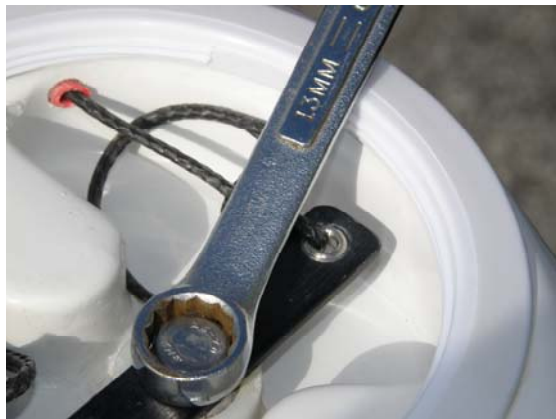
Photo 10. X-Series -- rudder removal – loosening 13 mm bolt
