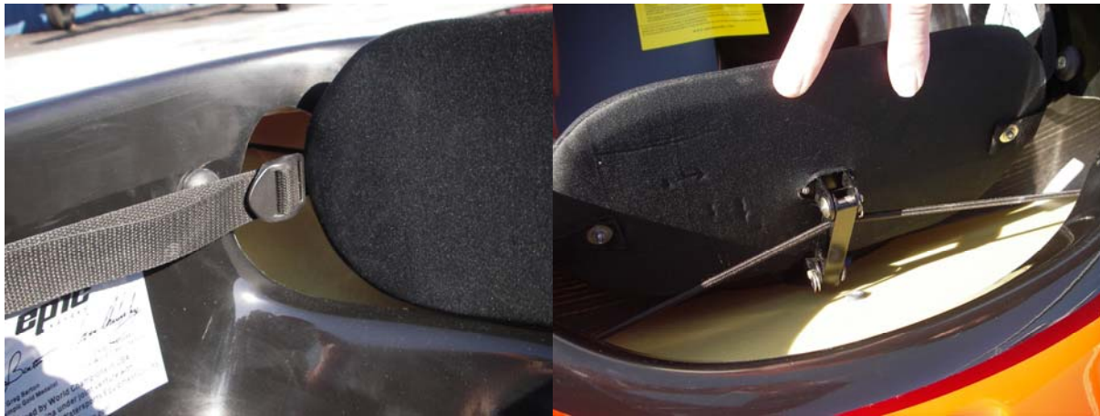
Photo 6. X-Series – straps and buckles for adjusting backband
