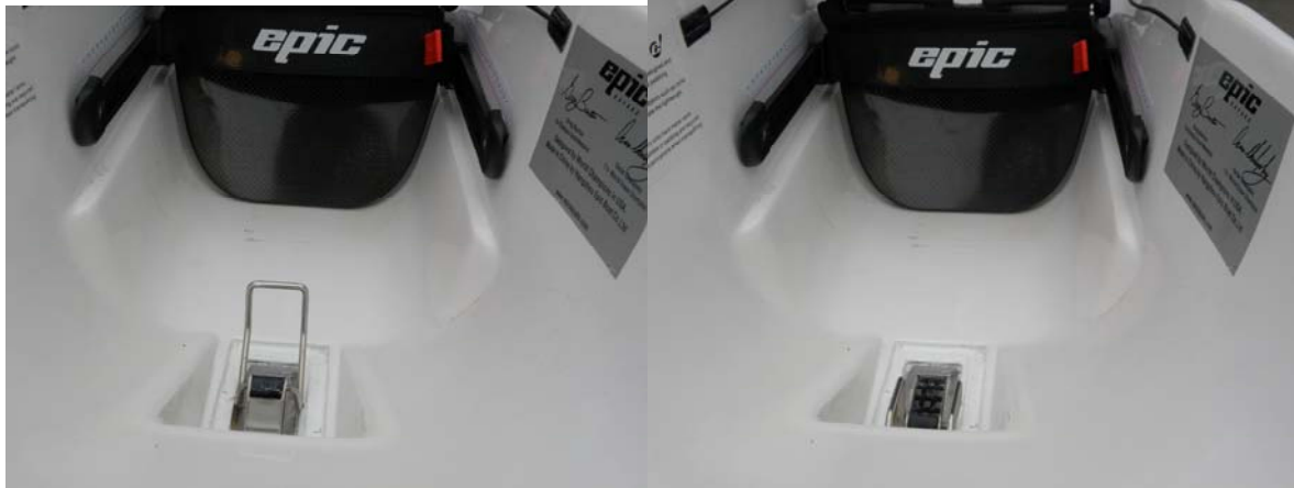
Photo 14. V-Series – bailer in position to open or close
