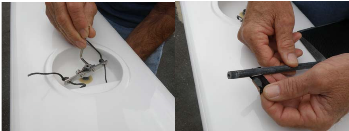
Photo 11. V-Series – loosen spreader bar assembly using allen wrench
